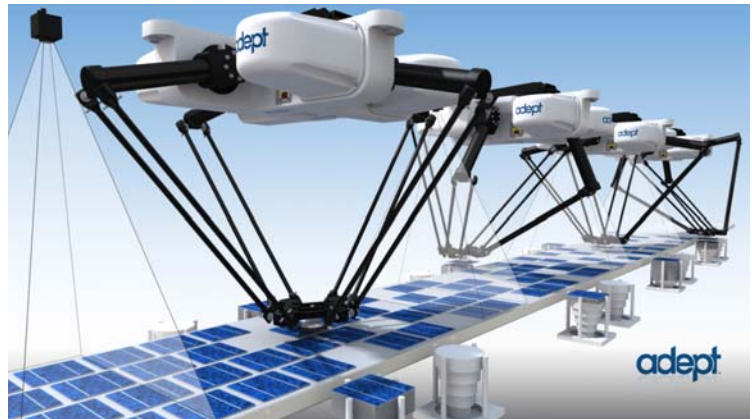
An AdeptSight image processing system controls several AdeptQuattro S650 robots handling solar cells
