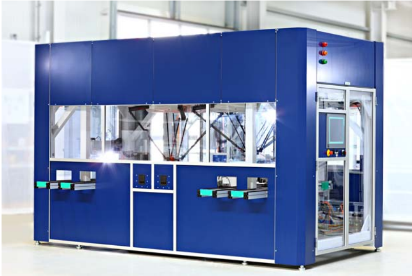
Two Adept Quattro s650 robotics systems in a cell handling solar wafers
